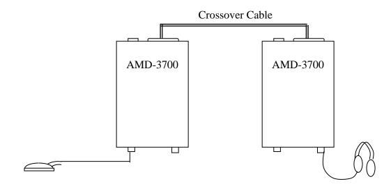
If sounds from the Chest Piece are heard at the headset, then the AMD-3700 units are working properly and if problems arise in connecting the unit to the Data Channel, it is appropriate to the concentrate on getting the signal through the Data Communications Channel.
