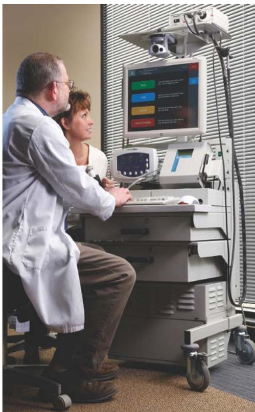
This fully integrated telemedicine cart\* is an all inclusive mobile telemedicine encounter work station with integrated medical peripherals, wireless network capability, and power management hardware that allows health care professionals to:
