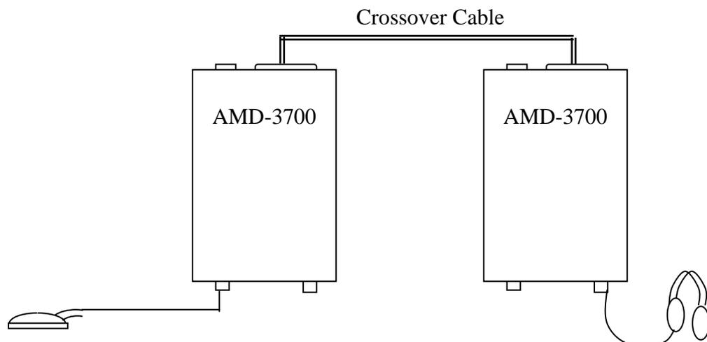
If sounds from the Chest Piece are heard at the headset, then the AMD-3700 units are working properly and if problems arise in connecting the unit to the Data Channel, it is appropriate to concentrate on getting the signal through the Data Communications Channel.
