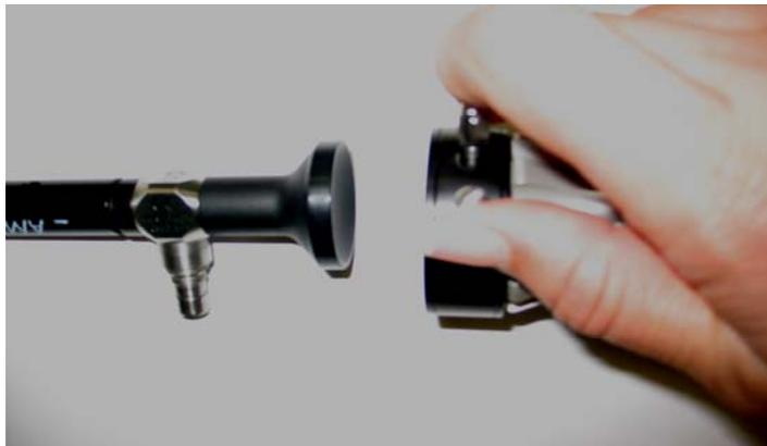
Simply slide the back of the AMD-2015 into the front of the AMD-2450. Make sure the scope sits even on the AMD-2450 coupler and close snaps to position.
