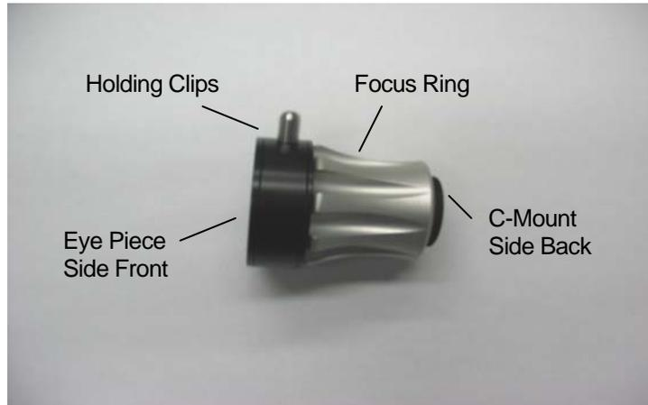
AMD-2015 ENT Scope – Components Diagram
